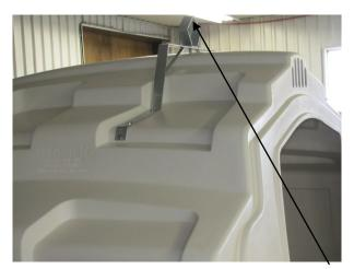
**Step#14** Install lift kit. Install top swivel first using 1/2" x 1 hex bolt with 1/2 nylon lock nut. Then place lift kit bracket as shown above. Mark and drill 3/8" hole in all 6 locations
