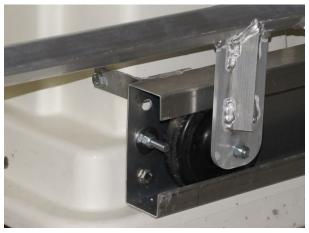
**Step#7** Insert wheel in side rail as **s**hown then install 3/8 nylon lock nut then tighten. Next install 3/8" x 1.5 hex bolt with two 3/8 flat washer on each side then install 3/8" lock nut. This bolt prevents the wheels from falling out of the side rails. Repeat this step on opposite side.
