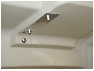
**Step#15** Install plate on inside as shown using  $3 \times 3/8$ " fender washer and  $3 \times 3/8$ " nylon lock nuts and tighten.
