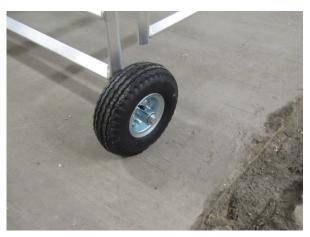
**Step#9** Install both front wheels to front feeding pane. Use 1/2" x 7 " hex bolt with 1/2" washer on both sides of the wheel housing then install 1/2" nylon lock nut and tighten.
