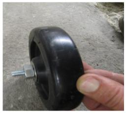
**Step#6** Install two 5" plastic wheels on support brackets on rear of side gate. Install one 3/8" x 3" hex bolt with 3/8 washer. Then on other side of wheel install 3/8" flat washer and 1/2 nut as spacer.
