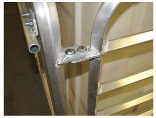
**Step#9** Install 4 x 3/8" x 1.5 hex bolts , 4 x 3/8" flat washers and 4 x 3/8" nylon lock nuts. Repeat this step on opposite side as well. Do not tighten until **Step#11**
