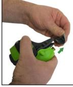
DO NOT force USB cable into port of unit. IMPORTANT: First charge should be overnight
