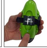
Do not turn unit off after calving (software updates are sent automatically over the GSM network and the sensor needs to be left powered on to receive same), only turn off the unit when storing for long periods.
